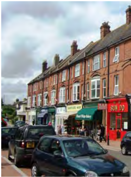
Towards the northern end, the High Street is strongly enclosed with the shops and houses set closer to the road with the 3 storey terrace of shops on the west side being the dominant feature. The red brick terrace has steep tiled roofs, regular chimneys just below the ridge and prominent bay windows under decorative brick arches on the middle storey, creating a rhythm of repeated patterns. The colourful but mainly traditional narrow shop fronts create a lively frontage. The terraced roofline is visible from Crow Hill and other vantage points in Borough Green.
